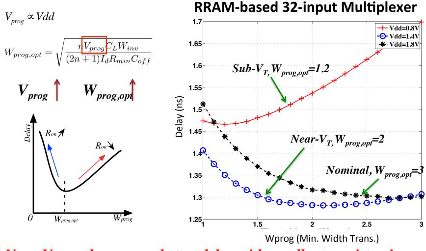
Near- $V_T$  produces even better delay with smaller transistor !
